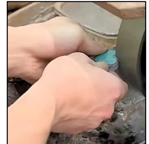
Step 4, Cut Left Side of Vee On Edge of Wheel
